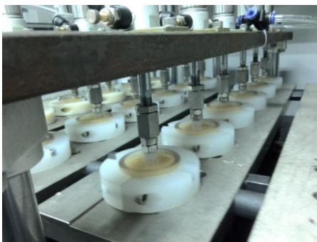
Figure 1: BiotriboPOD-Multi device designed and built up for the wear test of orthopedic biomaterials.
