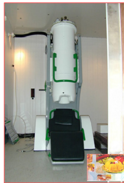
Figure 1: The 122-channel MEG system in the magnetically shielded room. One of the images for the visual stimulation (small icon).
